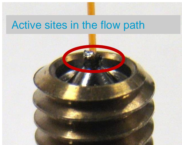
Extensive inlet maintenance needed
