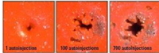
High-Temperature Septa Without CenterGuide: Major Coring Before 100 Autoinjections
